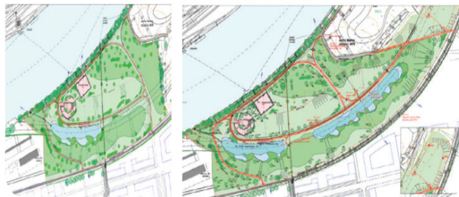
Fig. 15: Building No. 4679 Maniny – Prague Flood Prevention and Control Measures, decreasing the Karlín profile levelling baseline. Stage 0001 (a polder with a recreation/leisure zone) and stage 0002 (enlargement of a polder). Preparatory phase as of November 2016: final water management and building permissions have been issued Source: Water Management and Building, pls Prague
